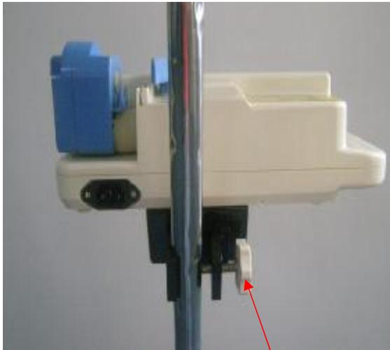
Rotate the other screw, make sure the syringe fixed on the IV stand
