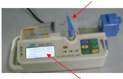
**The LCD displays the specification of injector**
