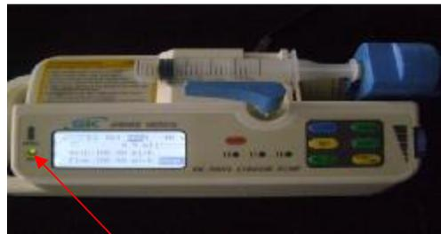
**The light is on, it means that the pump is in the state of charge.**
