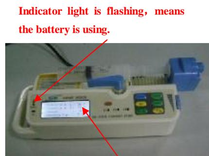
Indicator light is flashing, means the battery is using.
